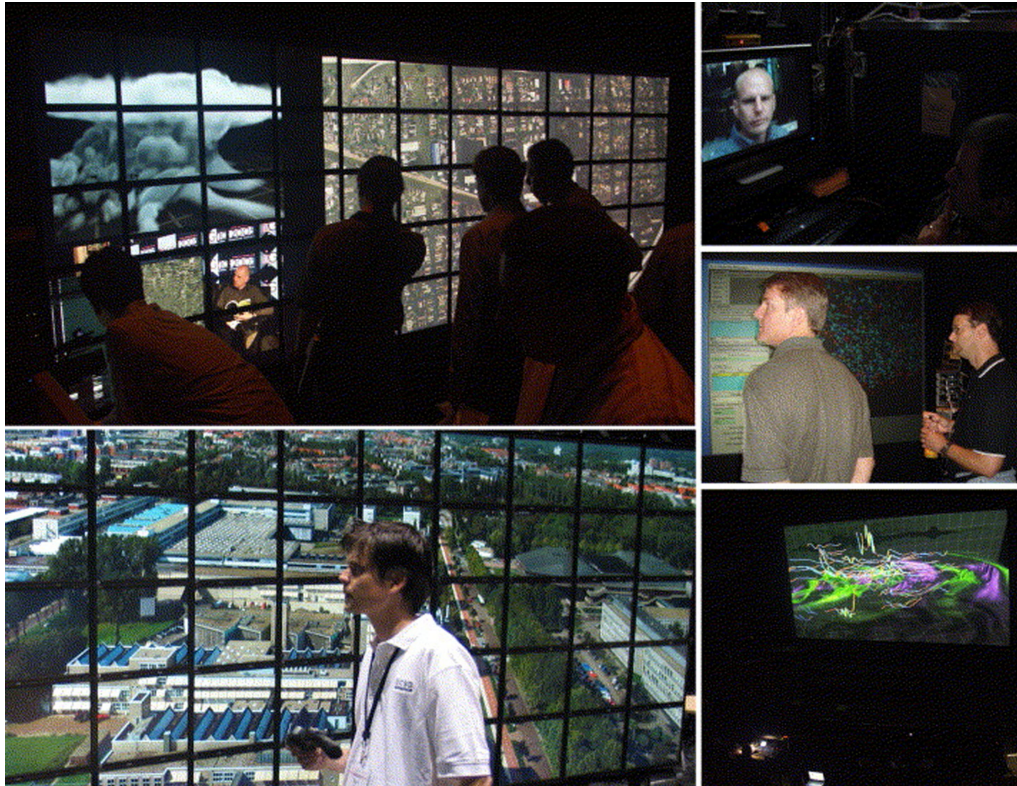
Figure 1. Visualization techniques shown during the iGrid2005 workshop: high-definition passive stereo displays (bottom right), auto-stereoscopic displays (top right), ultra-high definition tiled projection and LCD displays (left top and bottom)
