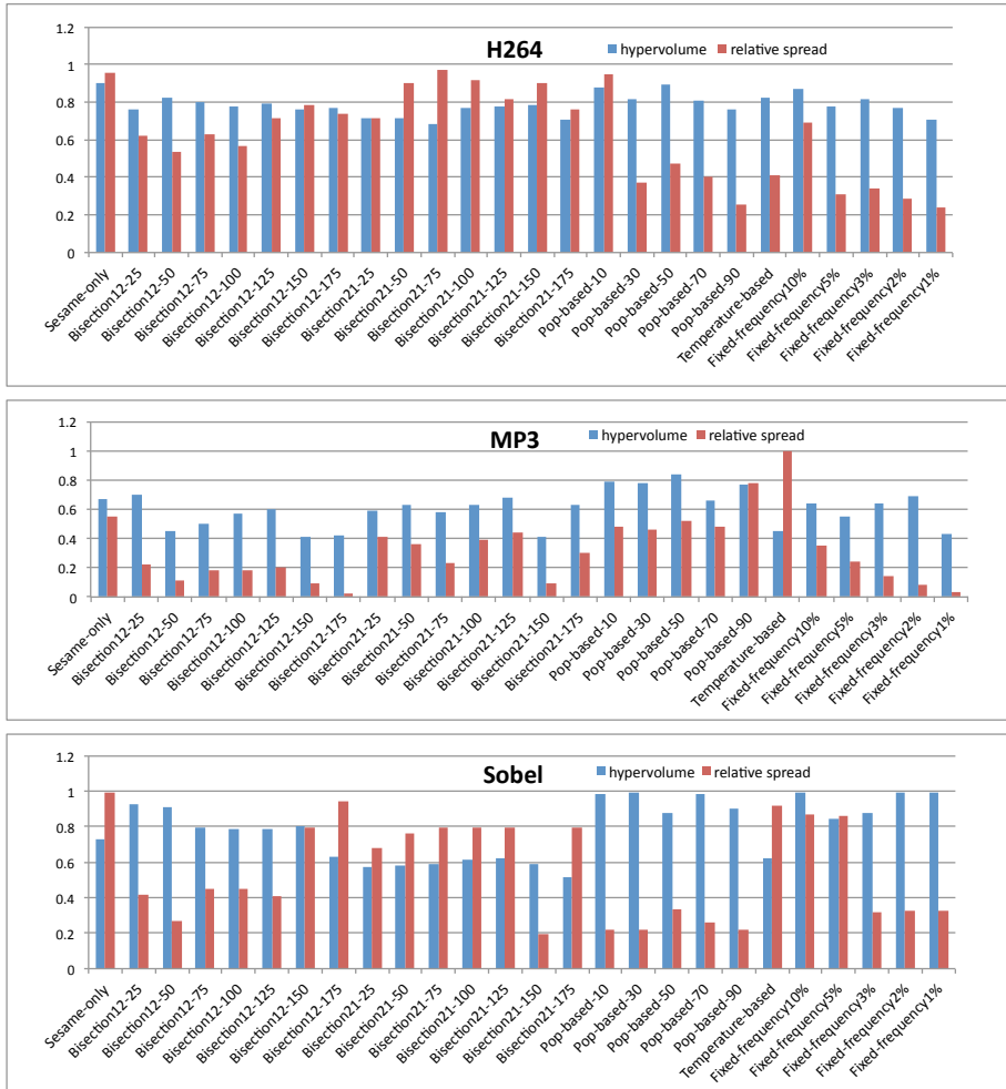
Figure 4.8: Average hypervolume and \nabla values for the different DSE methods applied to the Mp3 decoder, H264 decoder, and Sobel filter applications.
