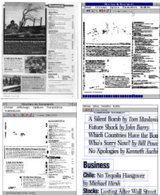
Figure 1: Physical Layout extraction by segmentation of text lines, binarization and bottom-up growing process
