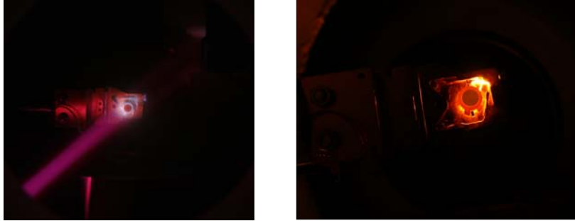
Figure 9: Left: Sputtering the gold test sample. With the lab light completely dimmed and the vacuum gauge turned off, the ion beam is visible as a bluish glow. Right: Annealing the gold test sample. The required current causes the connecting copper wires to glow brightly.
