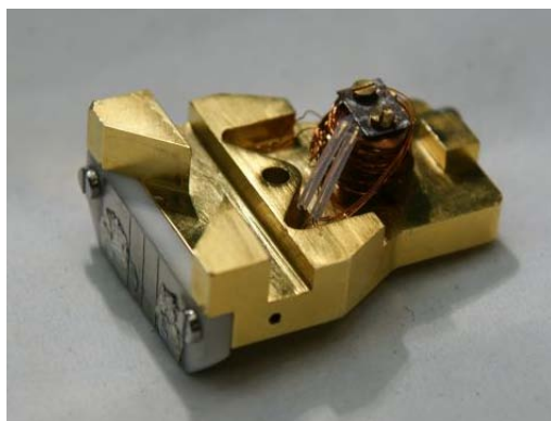
Figure 11: The sample used for the temperature calibration. The wound wire leads to the thermometer diode, which is held in place by the small metal plate.
