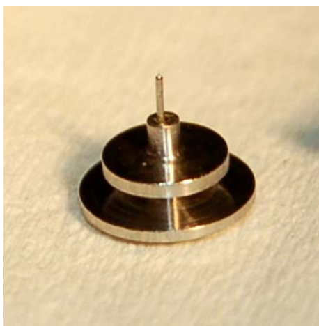
Figure 7: A tip. The tip itself is the thin wire sticking up from the center of the tip holder. The tip holder can be moved around in UHV by grabbing it with a fork that slides between the two discs of the tip holder.
