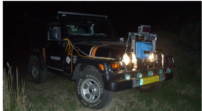
Fig. 1. RoboJep, TNO's research vehicle for autonomous navigation. The stereo cameras and the infrared spotlight are mounted above the headlights.
