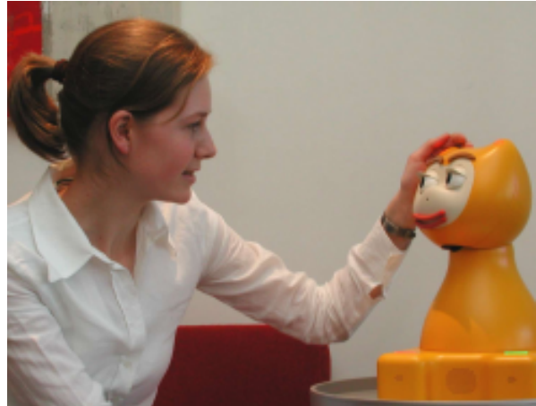
Fig. 1. Philips iCat interface robot [6]. The two microphones are mounted on the sides of the bottom panel.
