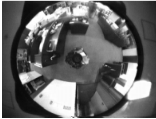
Fig. 1. Typical image from a camera with a hyperbolic mirror
