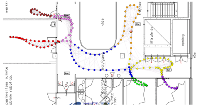
Fig. 5. The clustering found with the graph cut mechanism reflects the structure in the building
