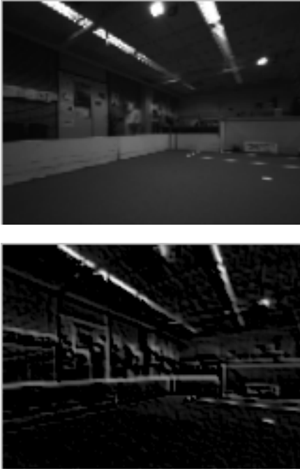
Figure 2: Plain image (top) and the same image after applying the Sobel filter (down).
