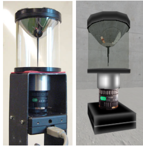
Fig. 1. The catadioptric omnidirectional camera, real and simulated.
