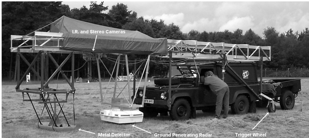
Figure 1. Picture of the LOTUS platform. A Land Rover vehicle has been equipped with a large aluminum frame, all the sensors are attached to this frame.
