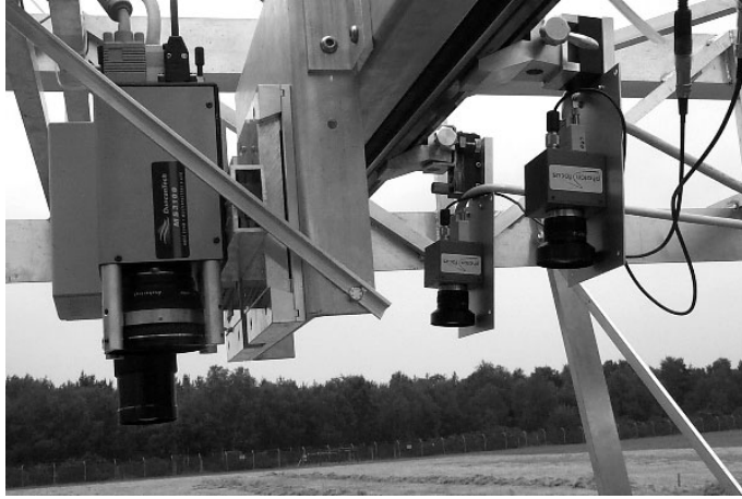
Figure 2. The picture shows the stereo cameras used for motion estimation. They were mounted near the other cameras which are used for gathering infrared and multi spectral data.
