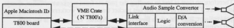
Figure 7. The ASC converts a digital signal supplied by a transputer to an analog signal. The ASC was developed at the electronics department of our faculty. [20] It consists of three parts, (1) a link interface, (2) logic to convert the byte wide link interface to the bit serial input of (3) the four times oversampling filter and digital to analog convertor (DAC). The ASC accepts 48000 32 bits words / sec. Each word consists of a 16 bit right- and left channel sample.
