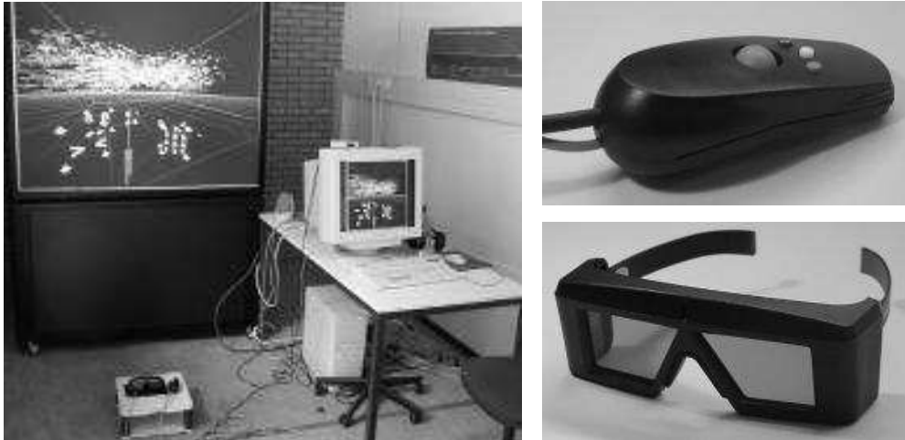
Fig. 13: DRIVE hardware, large screen, accompanying personal computer, wand, and shutter glasses. (images from UvA-DRIVE homepage, Belleman and Shukilov, 2003).
