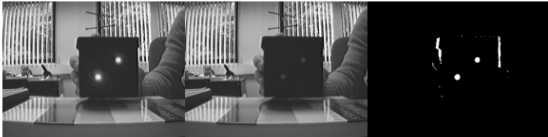
Figure 20. “Trails” produced by the movement of the device
