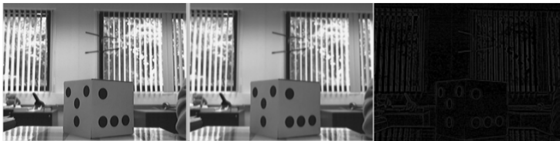
Figure 13. Noise reduction by Gaussian pyramid. Left: the original image, Middle: the smoothed image, Right: the amount of noise discarded
