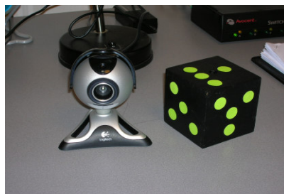
Figure 23. The device with color blobs and the Logitech QuickCam Pro 4000 webcam
