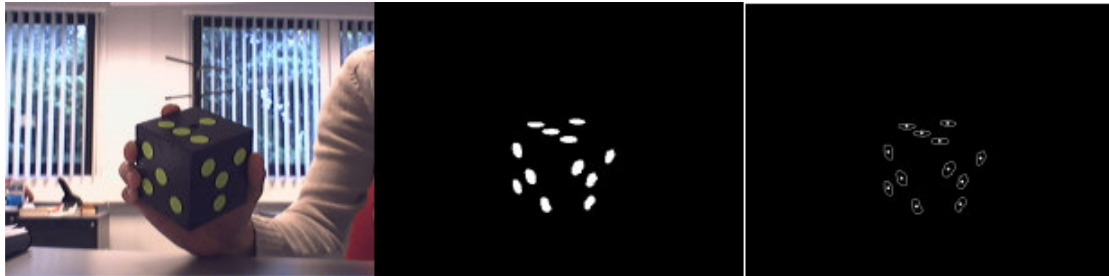
Figure 25. Experimental result. Left: the original color image, Middle: the image after color segmentation, Right: locations of the blobs detected
