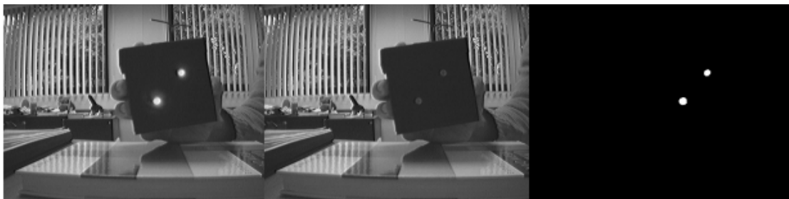
Figure 17. A pair of images in the expected case: LEFT: bright blobs, MIDDLE: dark blobs, RIGHT: blobs found after segmentation.
