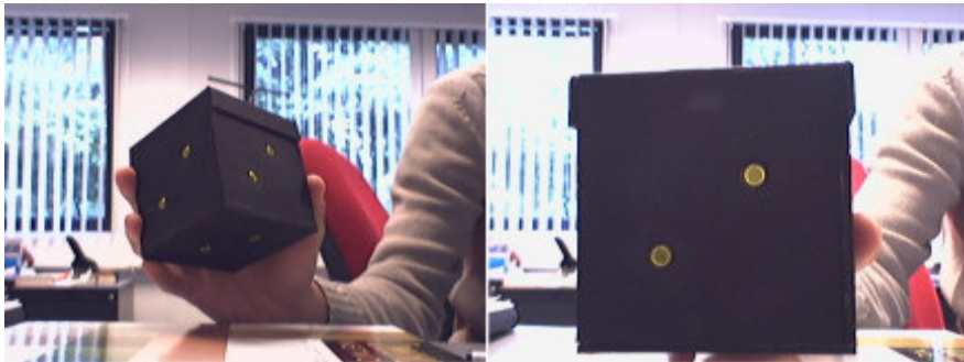
Figure 15. The cube device with active blobs and a close look at the LEDs
