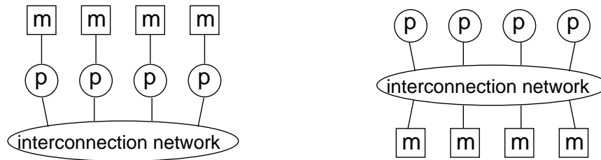
Figure 1.3: Distributed-memory and shared-memory parallel architectures.
