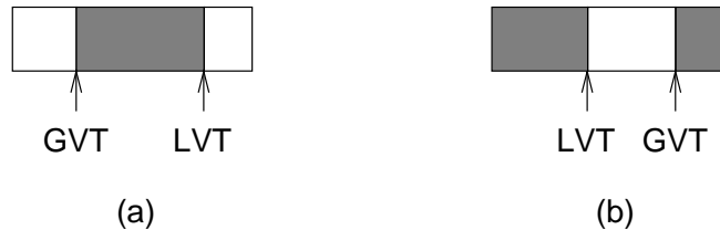
Figure 3.5: The circular I/O buffer for irrevocable operations. The two pointers GVT and LVT indicate the start and end of the buffered data. In (b) the LVT pointer swept past the circular buffer size.
