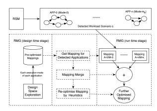
Figure 3: Mapping generation in the RMG component.
