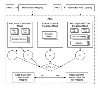
Figure 4: Overview of adaptive system reconfiguration in ARS
