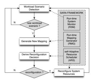
workflow of the SARA framework. When the RSM detects a new workload scenario, the RMG will generate a new mapping for the detected (active) scenario. Hereafter, the ARS makes an adaptation decision by predicting the benefit of changing the current mapping into the newly proposed one (by the RMG). According to this
