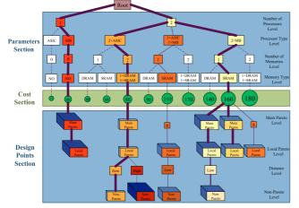
Fig. 2. Modeling the design space as a tree
