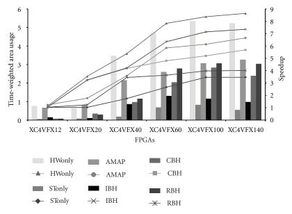
FIGURE 8: The comparison of different heuristics in terms of time-weighted area usage against speedup under different FPGAs conditions. The HWonly has the most time-weighted area usage, followed by the other runtime heuristics AMAP, CBH, IBH, and RBH.
