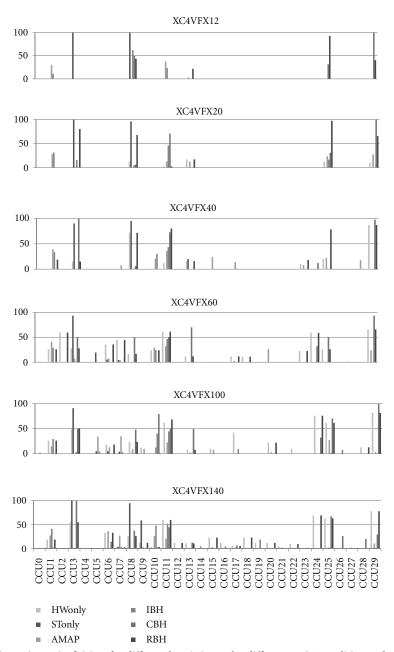
FIGURE 9: Reusability efficiency (RE<sub>Task</sub>) of CCUs for different heuristics under different FPGA conditions. The CCU reuse is significantly affected by the number of area slices in the FPGA.
