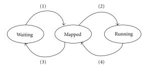
FIGURE 1: A finite-state machine (FSM) showing the different states of a task.
