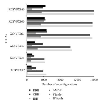
FIGURE 6: Heuristics comparison under different FPGAs conditions in terms of number of reconfigurations. There is a direct relation between the number of reconfigurations and the FPGA area.
