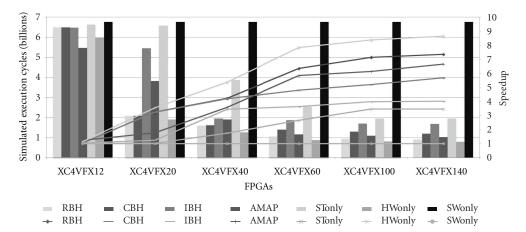
FIGURE 4: Comparison of the different heuristics tested in the proposed case study under different FPGAs conditions in terms of simulated execution time with corresponding application speedup. The application performance is proportional to the FPGA size. HWonly mapping has the best performance followed by RBH, AMAP, CBH, and IBH. STonly has the worst performance.
