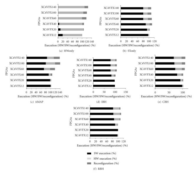
FIGURE 7: The comparison of different heuristics based on percentage of hardware execution, software execution, and reconfiguration. The hardware execution percentage is low in smaller FPGAs, and it increases considerably with more area slices.
