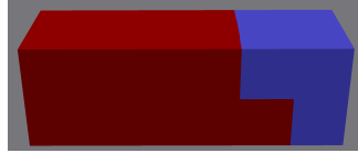
Fig. 3: Imbalanced domain distribution. Both the red and blue parts are assigned to half of the processes.
