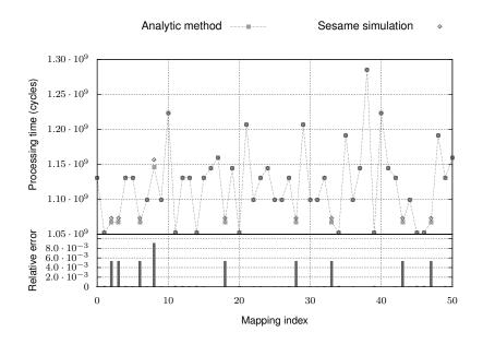
**Fig. 3.** Comparison between signature-based simulation and analytical models for M-JPEG mapping DSE on a crossbar-based multiprocessor architecture.
