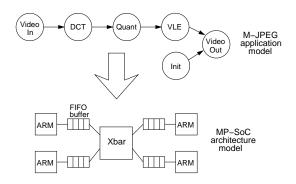
Fig. 2. Mapping an M-JPEG application to a crossbar-based MP-SoC architecture.
