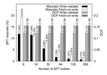
Figure 3. SPT missratio and DCP for a fetch-on-write and write-validate cache.
