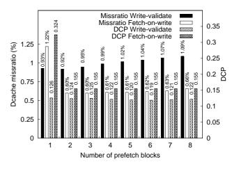
Figure 4. The performance when varying the number of prefetch cache blocks for fetch-on-write and write-validate.
