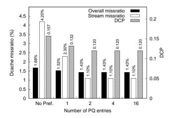
Figure 6. Performance of data-synchronised hybrid prefetching using a runahead of 3 and write-validate.
