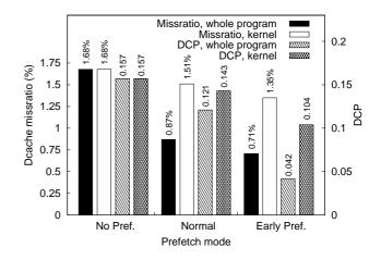
Figure 5. Performance of overall prefetching and kernel-only prefetching for write-validate, a 128entry SPT and an 8-entry PQ. The results of the early-prefetch optimisation are also shown.
