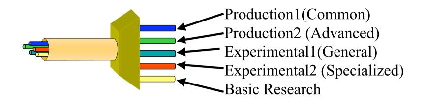
Eg, Experimental2 Could Be Provisioned From Remote Instruments In Other Countries Directly to University Labs – Finally, Separate Networks On the Same Infrastructure!
