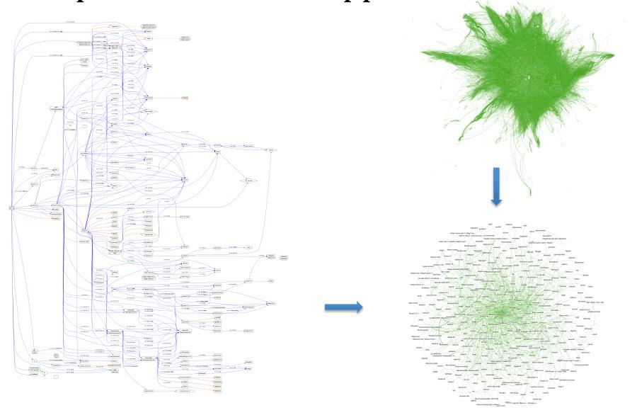
The application is fsl-4.1. LEFT: before dependency resolution, with all dependency constraints shown and RIGHT: resolved dependencies in a particular setup, libc is the center node
