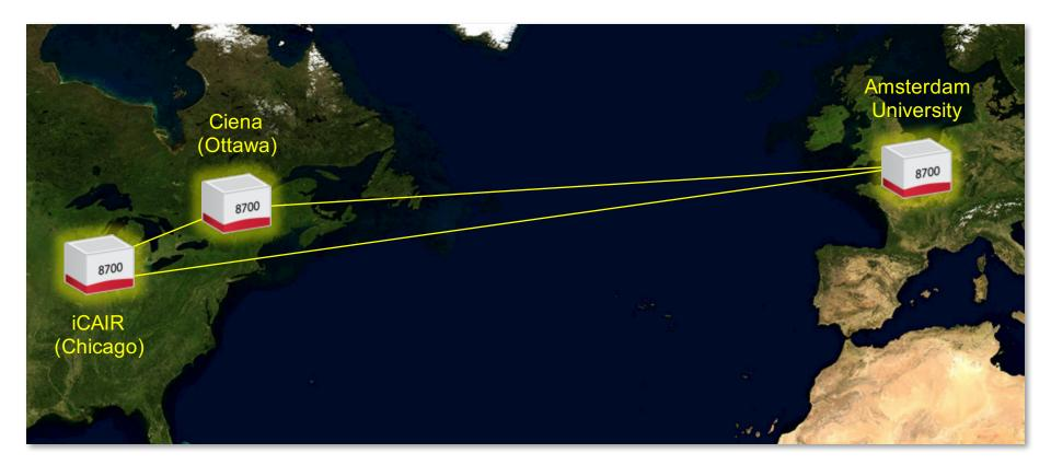
National Science Foundations ExoGENI racks, installed at UvA (Amsterdam), Northwestern University (Chicago) and Ciena's labs (Ottawa), are connected via a high performance 100G research network and trans-Atlantic network facilities using the Ciena 8700 Packetwave platform. This equipment configuration is used to create a computational and storage test bed used in collaborative demonstrations.
