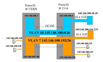
**Figure 4.** IP Addressing plan and VLAN configuration. This setup allows two type of paths. A switched 17 msec path and a 34 msec routed path.
