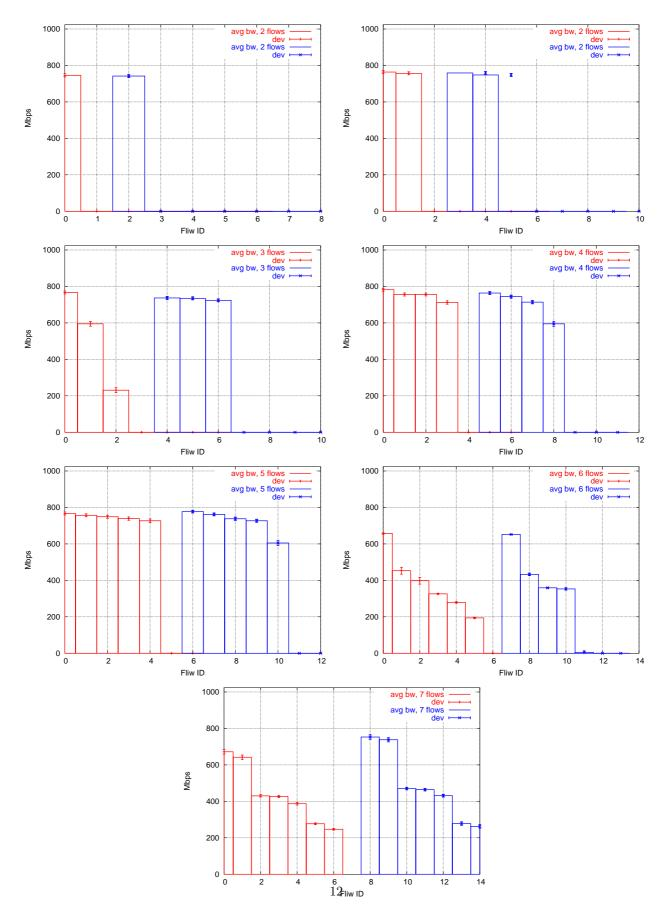
Figure 13. Average throughput of 25 minutes and standard deviation. The red lines denote the flows in one direction. The flows in the opposite direction are marked with blue lines. In this test the RTT between the sender and receiver node was 34 ms.
