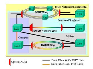
**Figure 1.** A possible scenario to use WAN PHY technology. 10 Gbps Ethernet can be used to interconnect networks over 2, 20 and 200 msec round trip in other words networks that span Metropolitan, National and International areas
