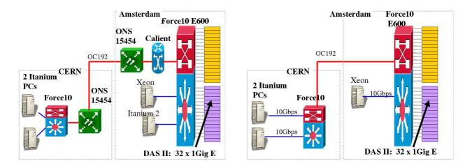
Figure 2. Setup using ONS The 10 Gbps switched network between Amsterdam and CERN, Geneva. The Lambda, SONET SONET OC192 Circuit, was terminated using 10 Gbps WAN PHY interface on the Ethernet Switch. At both ends Force10 switches were used.
