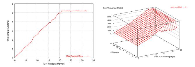
throughput vs socket size between Amsterdam and CERN. Throughput vs socket size and number of streams between Maximum throughput is is 5.22 Gbps CERN and Amsterdam
