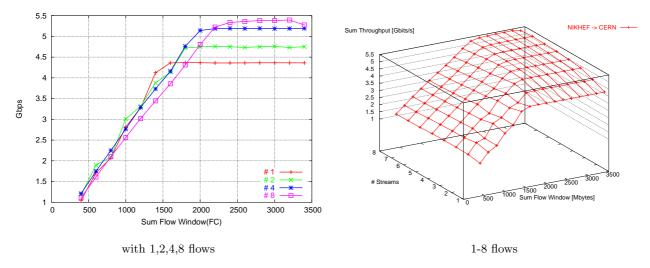
Figure 11. UDT memory to memory throughput vs FC and number of streams between Amsterdam and CERN, RTT = 17 msec
