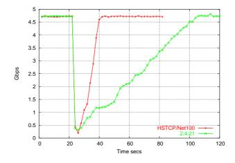
TCP congestion avoidance response. Throughput vs time for HSTCP and stock with 2.4.21 kernel
