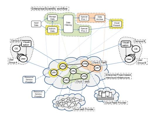
Figure 4. From scientific workflow to cloud based infrastructure.
