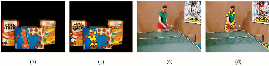
Fig. 2. (a) Example Soil data set and (c) frame from table-tennis sequence. (b) and (d) results of Harris detector (red dots) and the Harris detector with color boosting (yellow dots). The red dots mainly coincide with black and white events, while the yellow dots are focused on colorful points.
