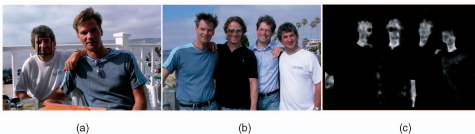
Fig. 6. (a) Training image depicting the region from which training data is obtained. (b) The image used for testing. (c) Signal-to-noise image.
